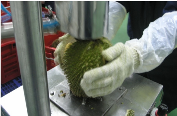
A mechanized durian opener ensures uniform and sanitary minimal processed products for export
